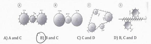
9. Which of the following diagrams of a motion transmission system correctly illustrates the motion of the components?
