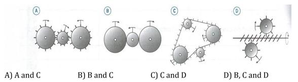
9. Which of the following diagrams of a motion transmission system correctly illustrates the motion of the components?
