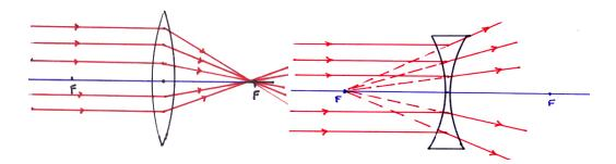
Primary focal point is after the lens in the convex lens And before the lens in the concave lens
